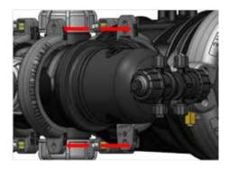
9. Remove the booster cylinder by pulling it backwards. Drain the booster cylinder from any water residue.
