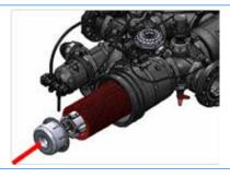
PLACE THE BUTTERFLY NUT ON TOP OF THE CYLINDER.
