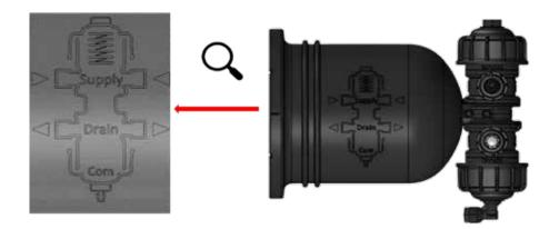
7. Disconnect the tubes of the water supply (S), water drainage (D) and command tube (C) from the booster cylinder (the location of the connection may be different for various configurations).
