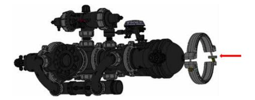
4. Keep pushing the cover while placing the upper clamp onto its location. Place the bottom clamp onto its location.
