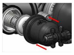
3. Place the system clamps around the booster cylinder.
