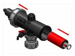
5. Wash the discs thoroughly under running water (make sure the discs are separated and spinning freely during the cleaning process).
