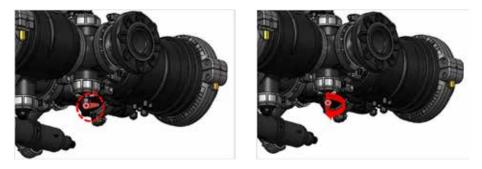
5. Open the command filter drain valve.
