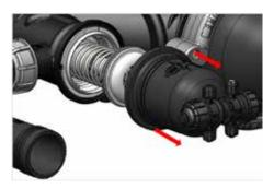
10. Reassemble the booster cylinder onto the flush valve.
