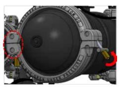
3. Push the bottom part of the main clamp downwards, making sure to support the cover during the procedure.
