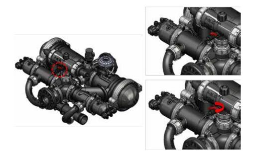
6. Disconnect the tubes of the water supply (S), water drainage (D) and command tube (C) from the booster cylinder.
