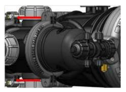
9. Remove the clamps (if needed, use a flat screwdriver to separate it).
