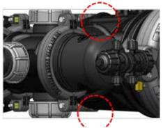
5. Connect the tubes of the water supply (S), water drainage (D) and command tube (C) to the booster cylinder.
