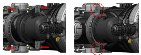
4. Tighten the two system clamps bolts by using a 13mm (1/2") spanner.
