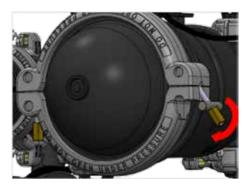
6. Tighten the two hex nuts (using a 17mm (11/16") spanner) that hold the main clamps together.
