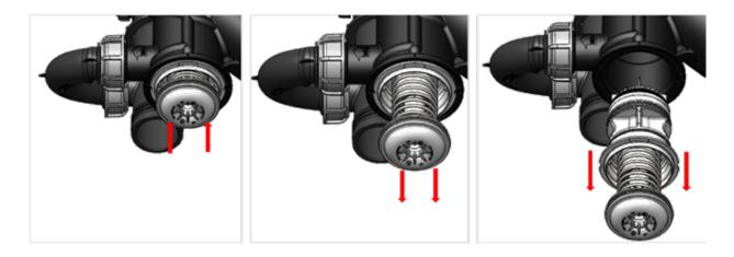
Visually inspect the valve for any signs of damage. Pay close attention to the seals.
