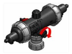
2. Reconnect the 8mm tube from the finger filter connection.
