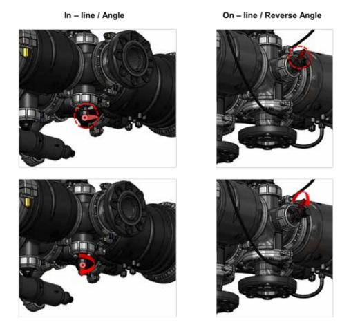
6. Open the command filter drain valve. In the On-line filter configuration, the drain is located at the bottom.
