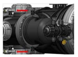
8. Remove the clamps (use a flat screwdriver to separate them if necessary).
