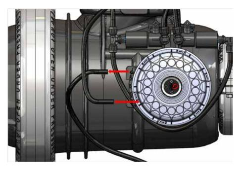
15. Disconnect the tubes that supply water to the solenoid, and leave unassembled, until next season.
