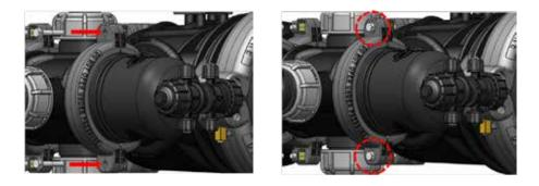
13. Connect the tubes of the water supply (S), water drainage (D) & command tube (C) to the booster cylinder.
