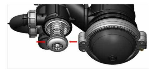
12. Push the piston valve forward and pull it back rapidly, until released
