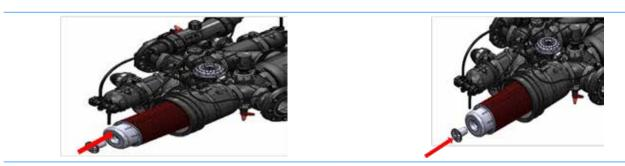
TIGHTEN THE BUTTERFLY NUT CLOCKWISE, USING THE PROVIDED TOOL.
