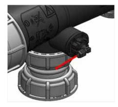
2. Rotate the finger filter counterclockwise (using a 30mm/1.2" spanner).
