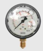
For the measurement of pressure and vacuum in irrigation systems, Netafim offers a wide range of pressure gauges with different pressure, filling and material. Pressure gauges are supplied with an air or glycerine filling (for signal damping) and with 1/4" bottom or rear connection.
