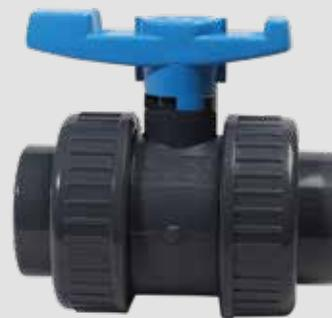
The TP ball valve is a compact manually actuated ball valve with single or double nut. The ball valve is characterised by a washer with screw thread. This makes precise adjustment of the ball seat possible. Furthermore, a washer with screw thread enables the outlet side to be removed when the ball valve is closed without the ball flying out of its seat.
