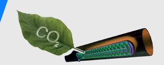
The Netafim labyrinths have a high mutual accuracy and unique properties. As a result, the labyrinth is also very suitable for use in emission systems for gases. The Aries Dose-line emission line is an inline dripline from Netafim specially selected for use with gas CO<sub>2</sub>.
