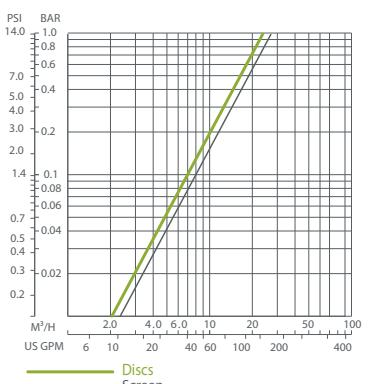
\*Pressure loss (with 'clean water and 130 micron screen)
