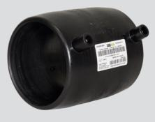
The SAB electrofusion welded fitting package is a limited package of PE electrofusion welded fittings for PE100 pipes. These economically attractive electrofusion welded fittings have a moulded-in heater coil that ensures welding of the fitting to the PE pipe as soon as voltage is applied. This results in a high-quality joint.
