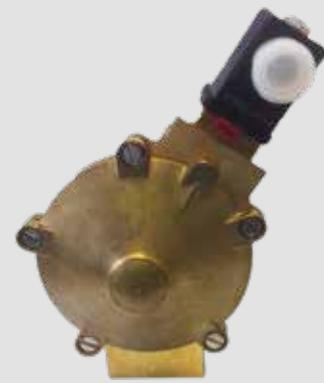
The Kentie diaphragm valve consists of a brass housing and cover, diaphragm and solenoid. The outlet side of the valve is on the side of the housing and has a female screw thread. The capacity opening is located in the middle on the underside of the housing and has the same female screw thread. The maximum working pressure is 10 bar. These angled diaphragm valves are available in the sizes 1", 1¼" and 1½".
