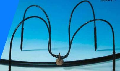
The CNL Multi-outlet is a combination of multiple Cobra drippers on a multi-outlet. The Multi-outlet is installed on a CNL dripper so that the Cobra stakes function practically like pressure-compensated and self-closing drippers.
