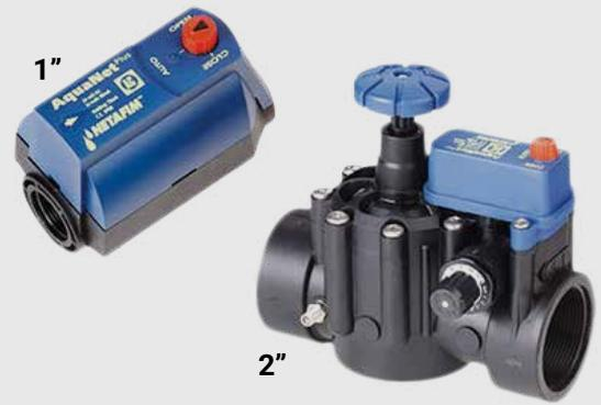
The AquaNet Plus valves are electric valves that are used for automatic irrigation of the garden and/or to divide it into various zones ("irrigation sections"). There are two models: 1" and 2". Both models are available in both AC and DC (latch) versions. The 2" valve has an integral pressure regulator (range 0.7 - 4.5 bar). All AquaNet Plus valves are also equipped with integral flow rate control and manual operation so that the AquaNet can be opened and closed independently of the controller.
