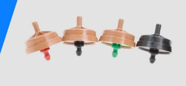
The CNL is a sturdy pressure-compensated and selfclosing dripper from Netafim suitable for the most difficult working conditions with contaminated water and large differences in height. The CNL has larger passages and higher closing pressures than any other dripper.
