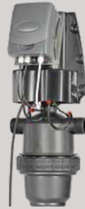
TAF filters are self-cleaning plastic filters from Amiad. TAF filters are based on the operating principle of the SAF family, but are tailored to smaller capacities. Only a small amount of flushing water is released during flushing. TAF filters are compact in design so that they can be easily installed. The filters are supplied complete with electronic differential pressure measuring, control (for pressure difference and/or time), with 230 V electric motor (or hydraulic motor) and drainage tap.
