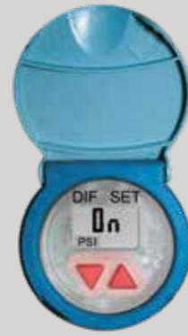
The Baccara differential pressure switch combines a pressure gauge and differential pressure switch in one unit that gives the user the freedom to program a wide range of monitoring and switching parameters for specific applications. This switch has been specially designed for the flushing of filters and enables a simple manual filter to be upgraded to an automatic filter. When the switch contacts are closed, the display shows: 'ON'.
