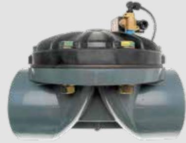
The Dorot 95/96 Series has a PVC housing with free passage and is therefore suitable for large capacities and/or low resistances. The function of the diaphragm minimises the risk of water hammer. Special soft diaphragms (low-flow) are available for applications with a minimum working pressure (0.5 bar).
