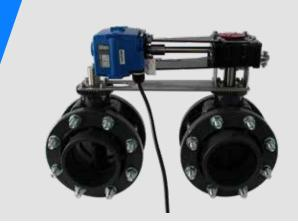
On the basis of the FIP-FE butterfly valves, Netafim has developed a number of double butterfly valves for the premixing of water flows, e.g. of rain or ditch water with decontaminated drain water. The valves are designed such that when one opens, the other closes at the same time so that good mixing of water flows is possible.
