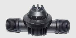
The Netafim DNL acts like a spring-loaded check valve that closes when the pressure in the system is relieved. The DNL prevents water from running back into lines and draining of lines that are installed with a slope or at different height, thus preventing differences in delivery.
