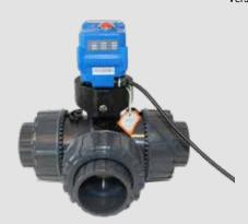
3-Way LKDIV ball valves can now be automated with a NedValve electric actuator, replacing a double operating pneumatic actuator. The L-model is supplied by default. Assembly with a NedValve or pneumatic drive is done using a Powerquick adaptor. The powerQuick adaptor is manufactured from PP-technopolymere (housing) and stainless steel shaft.
