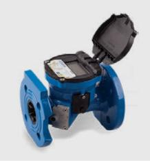
The Arad Octave is a revolutionary, accurate and reliable ultrasonic water meter based on the dual beam technology. The Octave has excellent hydraulic characteristics and advanced possibilities. Multiple output adapters are available for the Octave: double pulse (open collector, transistor), SSR pulse, analogue 4-20mA, ModBUS, SSR pulse + analogue 4mA.
