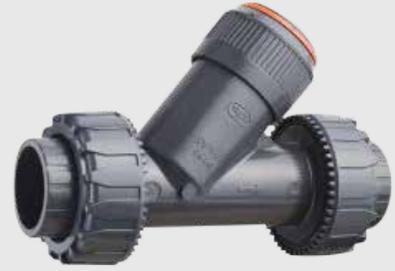
The FIP VRUIV check valve is a non-spring-loaded, removable valve with weight, in smaller diameters. This valve can be installed horizontally and vertically and can be employed with mechanically contaminated water in small waste water installations. Standard available in EPDM model. FPM O-ring sets are available separately. With proper use, the VRUIV offers a lasting leak-free connection.
