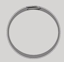
A special sprinkler pipe is the white sprinkler pipe for the installation of greenhouse sprinklers. These pipes have a thicker wall at the location of the threaded hole so that the sprinkler to be installed has more grip on the pipe wall.
