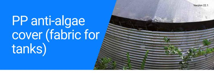
To limit the growth of algae, waves, heating, contamination and evaporation, Netafim supplies woven anti-algae covers that are fastened over the edge of the tank or float on the surface of the water.
