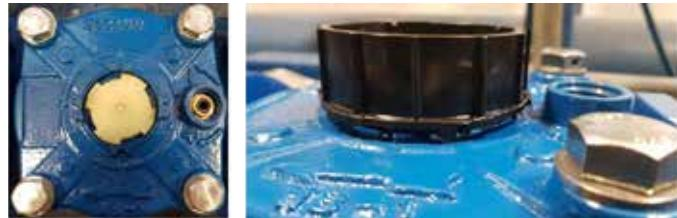
2) Line-up the register with the default flow direction, directing the 3 pointers on top of the calibration set screw
