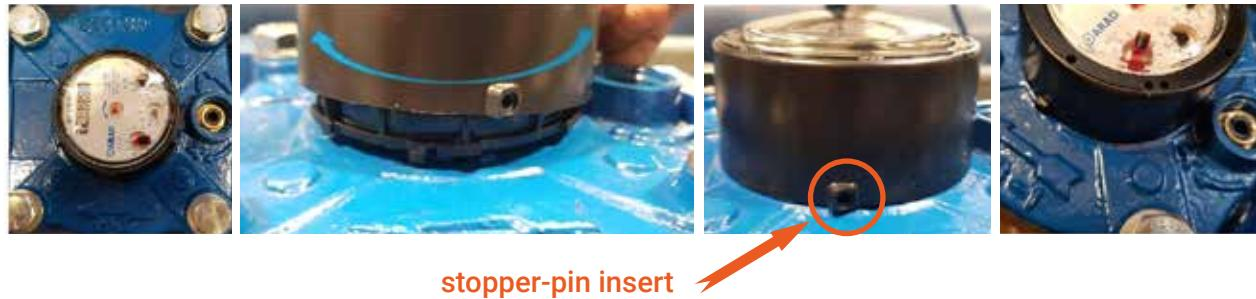
4) Insert stopper-pin in the outer housing and gently push through until the pin is completely inserted.
