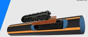
The UniRam RC is a pressure-compensated, non-self-closing inline dripline from Netafim. The pressure-compensated function of this product results in a very uniform flow rate even with longer lengths and/or small distances between the dripper points.
