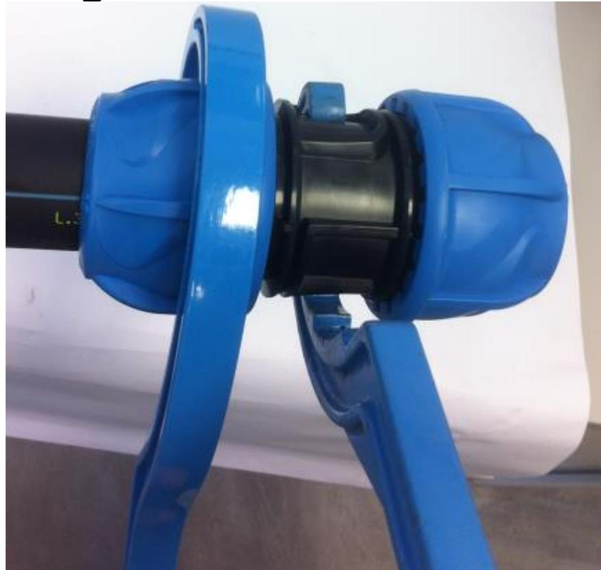
**DO NOT disassemble the fitting**
