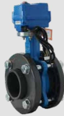
The ReValve metal butterfly valves are sturdy open/closed valves for various water processing and industrial applications. The butterfly valves have an epoxy-coated cast iron housing and stainless steel shaft with butterfly. The butterfly valves have a low torque. The valves can therefore be easily operated with a compact NedValve motor.
