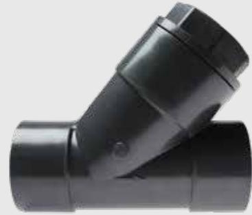
The FIP VRIV check valve is not spring-loaded, but is equipped with a weight. The valve cannot be disconnected. This valve is available in larger diameters. It can be installed both horizontally and vertically. Standard available in EPDM model. FPM O-ring sets are available separately.
