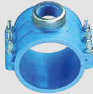
The tapping saddle from GF is recognisable from the blue colour and is used whenever a connection has to be made to an (existing) PE or PVC line with a diameter from 20 to 315 mm. 654X has KIWA certification and is used in particular for drinking water lines and in the agricultural sector.
