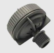
Just like the line flushing valve, the air vacuum breaker valve helps cleaning of driplines by creating a vacuum in driplines to prevent from dirt entering.
