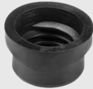
The installation ring is used for installing sprinklers in, for example, aluminium irrigation lines. Screwing the sprinkler into this ring causes the ring to expand and to be clamped firmly in the drilled hole. This ring can also offer a solution when the screw thread of the sprinkler in the irrigation line is damaged.
