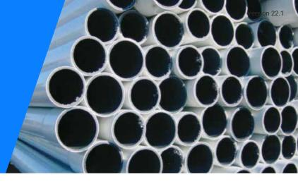
White PVC pressure pipe is produced by co-extrusion of white (outer layer and dark grey (inner layer) raw materials. This pipe has maximum light reflection, resulting in a lower water temperature and hence less growth of algae in the pipe. The pipe has a moulded adhesive insert and a chamfered end for easier gluing.
